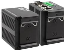
The wall bracket can be mounted using the same threads as the DIN-Rail Kit
