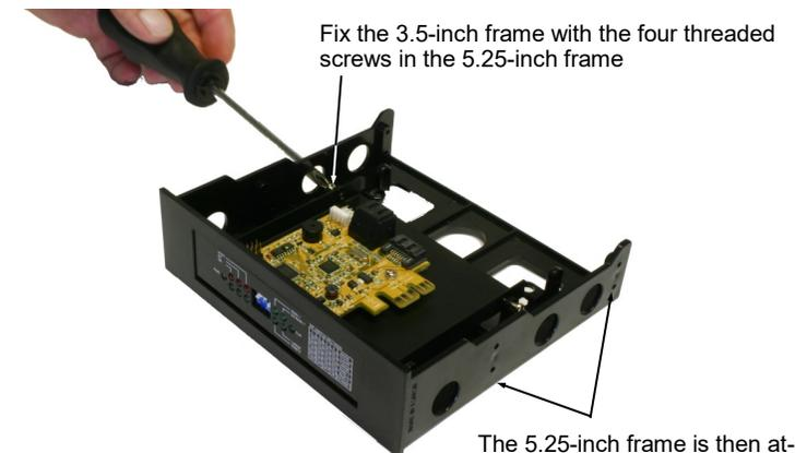
Fix the 3.5-inch frame with the four threaded screws in the 5.25-inch frame
